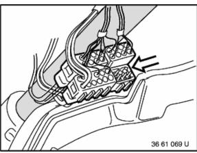
Loosen cable straps on steering column. Disconnect plug connection.
