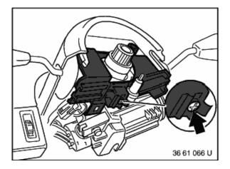
Remove screw for holder of steering-column stalk.
