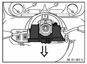
Lever off holder in downwards direction using a screwdriver.
